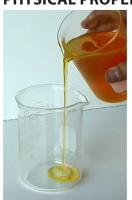
Boiling point:>473°F (>245°C)Specific Gravity:1.04 - 1.08 (Kg/Liter)Weight per Gallon (US):8.66 - 9.00 (lbs/gal) (US)Appearance:Viscous, orange tinted liquid
